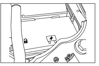
The engine compartment fuse block is located on the driver's side of the engine compartment. See *Engine Compartment Overview on page 5-12* for more information on location.
